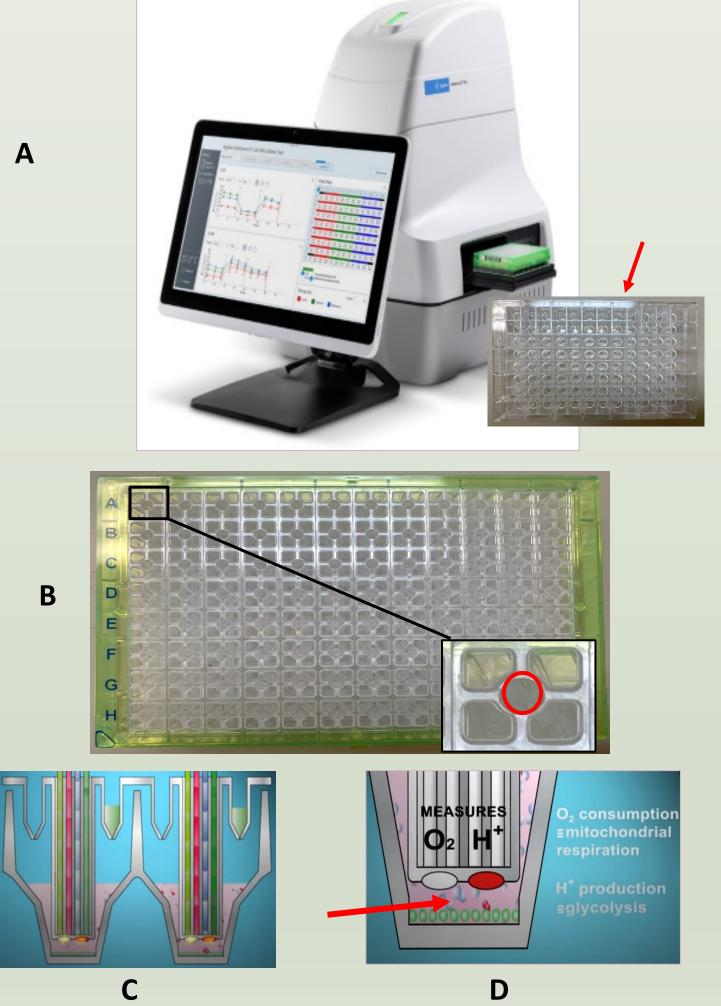
Figure 1. The schematics and principle of Seahorse analyzer
